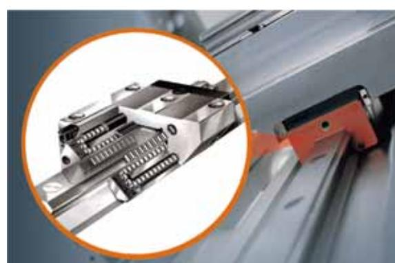
Roller-type LM Guide is mounted on the machine to improve rigidity and feedrates. Each axis is powered by a maintenance free digital AC servo motor. These high torque drive motors are connected to the ball screws without intermediate gears for quiet and responsive slide movement with virtually no backlash.
