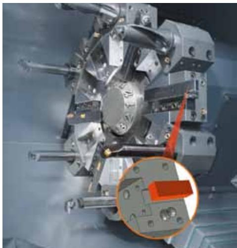
heavy duty turret features a large 210mm diameter curvic coupling and 39 kN of hydraulic clamp force. The heavy duty design provides unsurpassed rigidity for heavy stock removal, fine surface finishes, long boring bar overhang ratios, and extended tool life.
