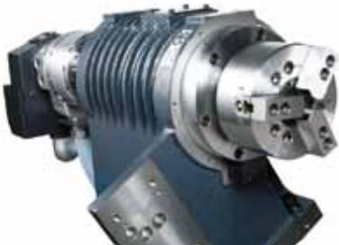
The headstock and main spindle are manufactured in a temperature controlled environment then assembled and tested in our clean room. The heavy duty cartridge type spindle is supported by a triple row angular ball bearing in the front, with a row cylindrical roller bearing in the rear. This combination of bearings is very effective in refraining from thermal displacement of its front nose and improving high speed performance and its rotational precision.
