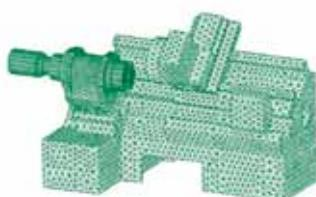
FEM analysis used to design a stable body.
