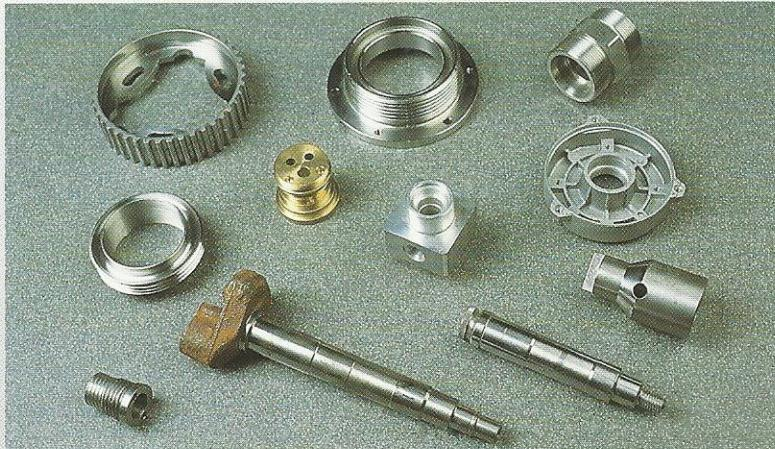
MILLING, DRILLING, TAPPING
