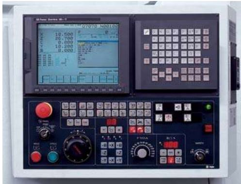
CNC Fanuc 31 i-T con video a colori 10.4" a cristalli liquidi CNC unit mod. Fanuc 31 i-T, 10.4" colour liquid crystal display
